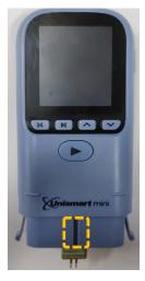
Ensure that the JIG's alignment groove and the device's screen are on the same side.
